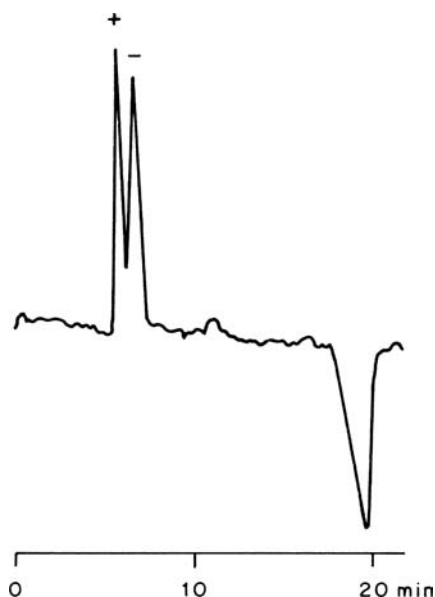
Figure 22.2 Separation of N -(1-phenylethyl)phthalamic acid enantiomers with a chiral ion-pair reagent [reproduced with permission from C. Pettersson, J. Chromatogr. , 316 , 553 (1984)]. Conditions: stationary phase, LiChrosorb SI 100, 5 \mu\text{m} ; mobile phase, dichloromethane–butane-1,2-diol (99 : 1) containing 0.35 mM each of quinine and acetic acid; UV detector. The negative peak at ca. 19 min is a system peak.
