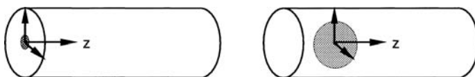
Figure 2.4 Band broadening by longitudinal diffusion. Left: Sample zone immediately after injection. It will spread out in all three axes of space (arrow directions). Right: Sample zone at a later moment. It is larger now due to diffusion and it has also been transported by the flowing mobile phase.
